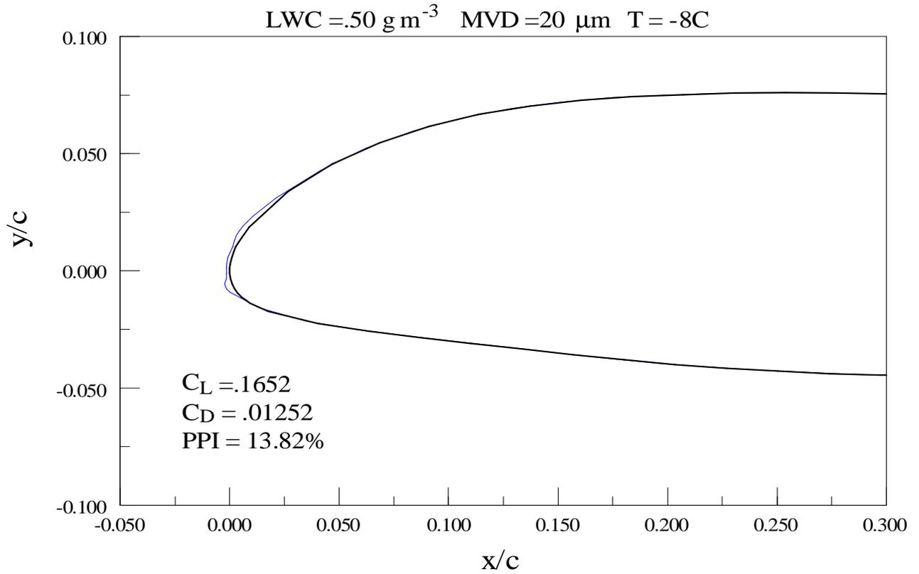
**Figure 1.** The chord cross section of a five minute ice accumulation (blue) on a 1.5 m NACA 23012 airfoil moving at 90 m s<sup>-1</sup> with meteorological conditions noted at the top. The axes are labeled as a fraction of chord length from the leading edge.  $C_L$  is the resultant coefficient of lift.  $C_D$  is the resultant coefficient of drag. The accumulated ice results in a 13.82% power increase (PPI) needed to maintain speed and altitude. See McCann (2004) for details.
