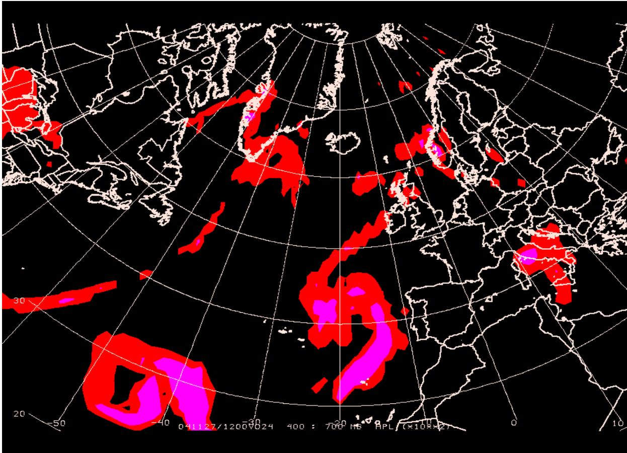
**Figure 2. VVICE forecast of the maximum aircraft icing in the layer from 700 mb to 400 mb (FL100 to FL240) from the 24-hour Global Forecast System numerical model verifying at 1200 UTC, 27 November 2004, over the north Atlantic Ocean region. The red areas are greater than 10% percent performance loss (PPI) and the magenta areas are greater than 60% PPI.**
